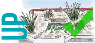
Raised overflow units are often used to help keep stormwater in the landscaped area so it can infiltrate naturally into the soil.
