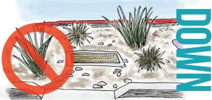
When not properly elevated, runoff merely goes "down the drain." When designing or constructing a stormwater landscape, make sure overflows are set at the proper elevation.
