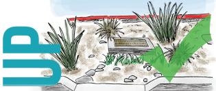
Raised overflow units are often used to help keep stormwater in the landscaped area so it can infiltrate naturally into the soil.
