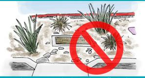
When not properly elevated, runoff merely goes "down the drain." If you are designing or constructing a stormwater landscape, make sure that overflows units are set at the proper elevation.
