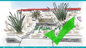
Raised overflow units are often used to help keep stormwater in the landscaped area so it can infiltrate naturally into the soil.
