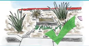
Raised overflow units are often used to help keep stormwater in the landscaped area so it can infiltrate naturally into the soil.
