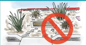
When not properly elevated, runoff merely goes "down the drain." If you are designing or constructing a stormwater landscape, make sure that overflows units are set at the proper elevation.
