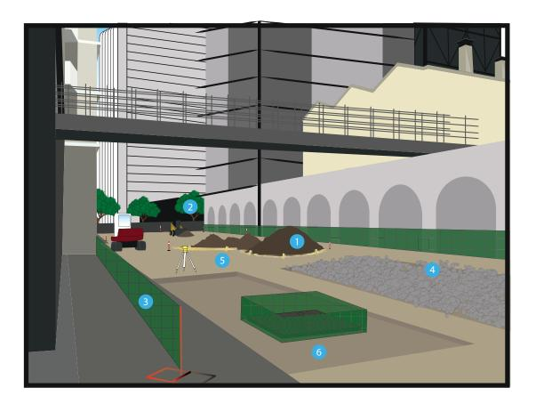
STOCKPILE MANAGEMENT- Cover and protect excess site materials, provide perimeter protection. See Section 5.5
