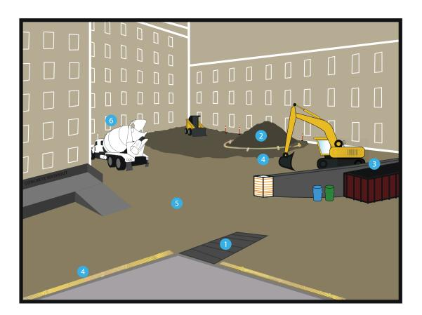
STABILIZED CONSTRUCTION ACCESS - Install rock pad, mat or rumble plates at entrance to site to prevent tracking of soils onto nearby streets. See Section 3.1
