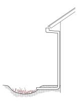
Connecting a roof leader to a vegetated area. The head from the eave height makes it possible to route roof drainage some distance away from the building.
