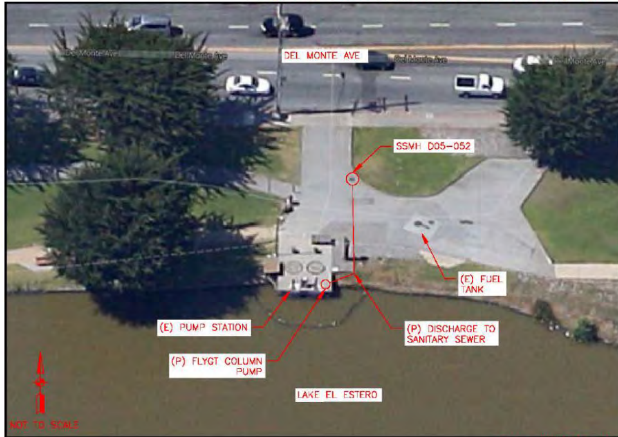
Figure 3 - Lake El Estero Water Intake Pump Option
